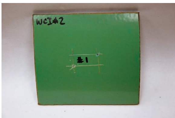
Figure 2. NACE RP0394 Hot Water Soak Test, number 1 rating.
