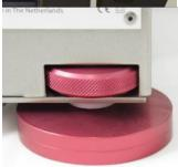
Design 'Solid Supports' to level the instrument.
