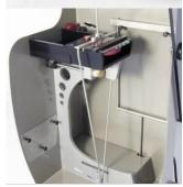
Integrated storage of glass plate and pendulum.
