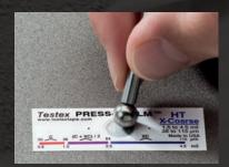
For use with Testex™ Press-O-Film™ Replica Tape
