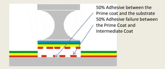
50% Adhesive between the Prime coat and the substrate
