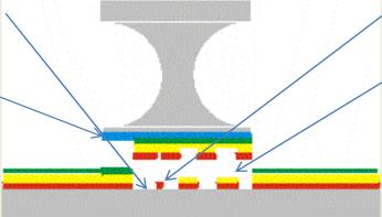
5% Adhesive split between the Prime Coat and the intermediate coat 30% Cohesive failure in the Intermediate coat
