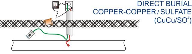
Model DB-A Copper-Copper/Sulfate Reference Electrode designed for direct burial for long term monitoring of buried or earth contacting structures.
